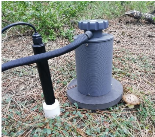
Figure 9. Trenching excavation (top left) and refilling work (top right) in autumn 2021, and respiration measurements being carried out with EGM-5 CO 2 analyzer (PP-Systems) on inserted collars during the 2022 campaign (bottom).
