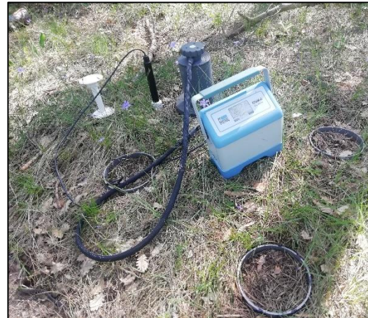
Figure 9. Trenching excavation (top left) and refilling work (top right) in autumn 2021, and respiration measurements being carried out with EGM-5 CO 2 analyzer (PP-Systems) on inserted collars during the 2022 campaign (bottom).
